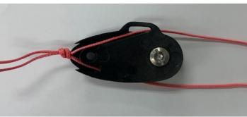
The cord must be thread through the side opposite of the spool and secured with a slip knot.
