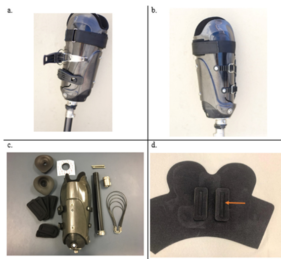
Fig 1 Components of the immediate fit prosthesis. (A) Lateral view of prosthesis displaying locking buckle system; (B) medial view of prosthesis displaying hooks used to make fine adjustments to the socket's circumference; and (C) the “prosthesis in a box” kit including a socket, neoprene liner, padding kit, spacers, adhesive, pylon, tube clamp, pins, and various sized cables. All that is needed in addition to the kit is a sleeve with pin attachment (pins are included) for suspension and a prosthetic foot. (D) A 5-mm perforated neoprene liner shown with additional pads (arrow) that stick to the liner with velcro and can be placed to relieve socket pressure and reduce discomfort. These pads allow for a customized socket fit.
