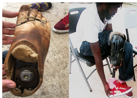
Fig 2 The prosthetic foot (left) showing breakdown of the outer cover after 6 months of use. The iFIT socket (right) remained in working order over 7 months after being used extensively while performing this individual’s occupation (agricultural work).
